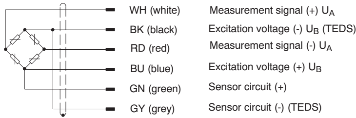
Cable shield, connected to housing
